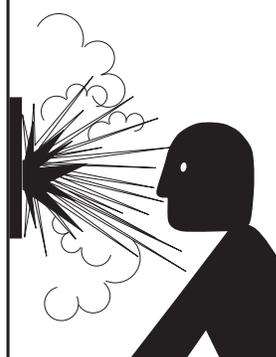
Manually operate the temperature and pressure relief valve at least once a year to make sure it is working properly. To
