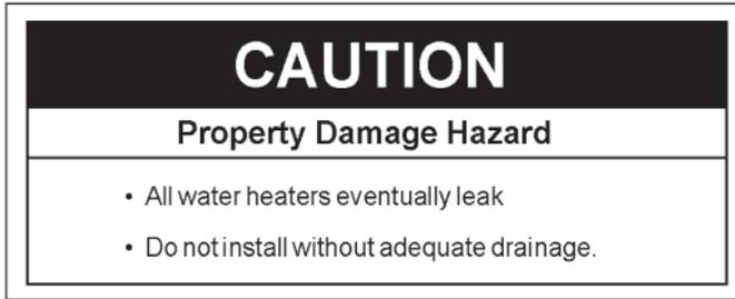
It is always recommended that a suitable metal drain pan be installed under the water heater to protect the area from water damage resulting from normal condensation production, a leaking tank or piping connections. Refer to the "Site Location" section.
