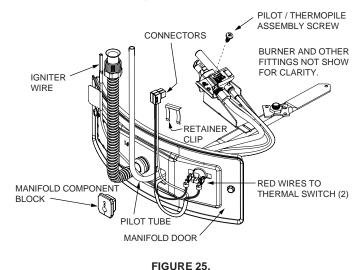
6. Read this step carefully before proceeding. Using the old pilot/pilot tube assembly as a guide, bend the new pilot tube to match the old one. Make only the bends closest to the pilot before going to the next step.
