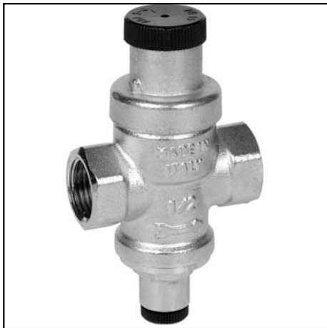
Figure 15 - A Pressure Reducing Valve is required if your home's water pressure is above 80 psi.
