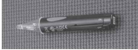
Figure 25 - Non-Contact Circuit Tester
