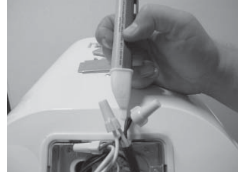
Figure 28 - Non-Contact Circuit Tester
