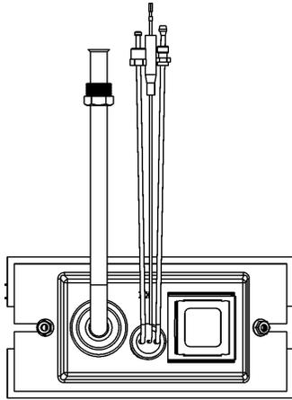
Figure 4. BURNER ASSEMBLY PARTS
