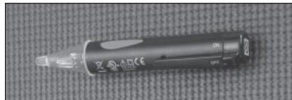
Figure 31 - Non-Contact Circuit Tester
